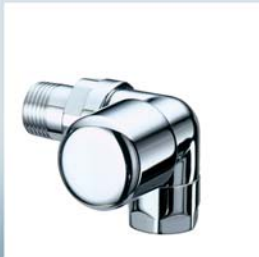
Art. 0101 Thermostatic valve, angled-left version - Interchangeable sizes for copper, plastic and multilayer pipe - Size: 3/8" - 1/2" - Installation: water supplied to radiator
