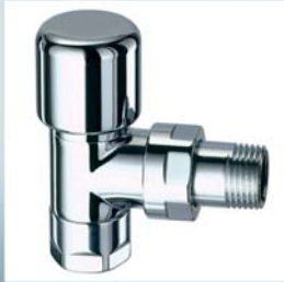
Art. 0108 Thermostatic angled valve - Interchangeable sizes for copper, plastic and multilayer pipe - Size: 3/8" - 1/2" - Installation: water supplied to radiator
