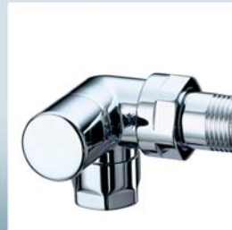
Art. 0122 Lockshield valve, angled-right version - Interchangeable sizes for copper, plastic and multilayer pipe - Size: 3/8" - 1/2" - Installation: returned water from radiator
