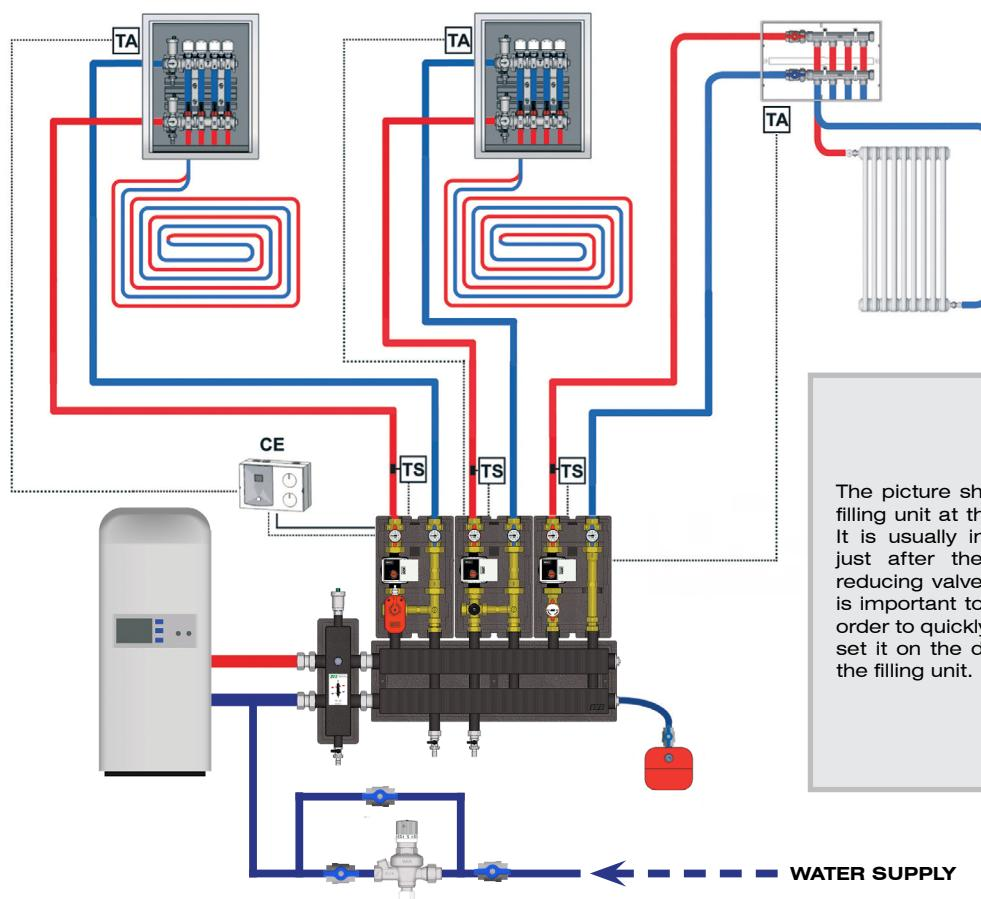
The picture shows a typical installation of a filling unit at the inlet of the heating system. It is usually installed on the return circuit, just after the strainer and the pressure reducing valve. As previously mentioned, it is important to have a bypass on the unit in order to quickly fill up the system and then to set it on the desired calibration value using the filling unit.
