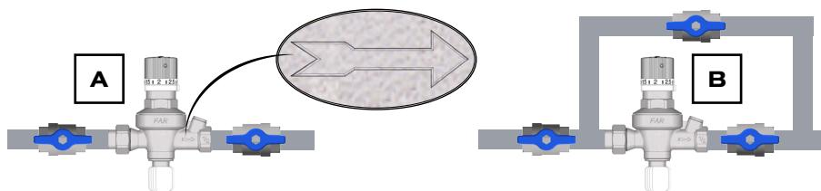
**⚠ The filling unit can be installed in a horizontal or vertical position, but not upside down.**
