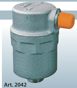
Fig.1 - If there is no air in the circuit, water inside the air vent valve keeps the float in such a position as to close the shutter.
