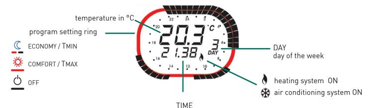
The program setting ring shows a 24-hours clock, divided into 30 min sectors. The sector colour indicates the set temperature for that period.
