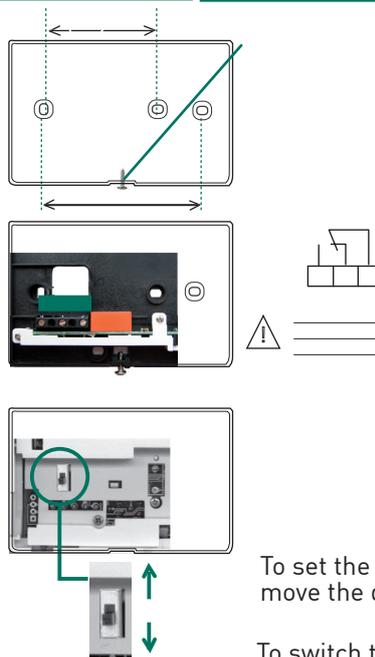
To set the ANTIFREEZE 5°C protection move the dip switch HIGH.
