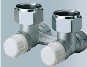
Art. 1422 SINGLE-DOUBLE PIPE angled valve. Adjustable by-pass. Connections: FAR 24 x 19 Centre line between ports: 50 mm
