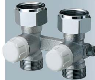
Art. 1422 SINGLE-DOUBLE PIPE angled valve. Adjustable by-pass. Connections: FAR 24 x 19 Centre line between ports: 50 mm
